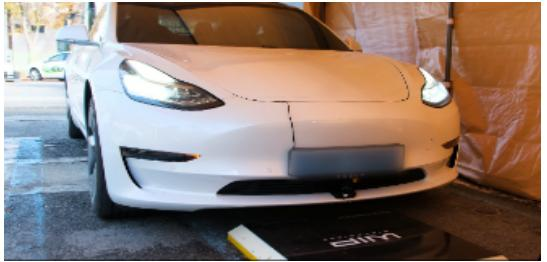
A white Tesla Model Y electric vehicle connected to a charging pad on the ground. |
